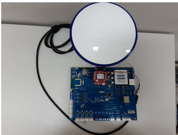
[Figure 6] Design circuit diagram of proposed settlement detector based on microprocessor board and gnss module
