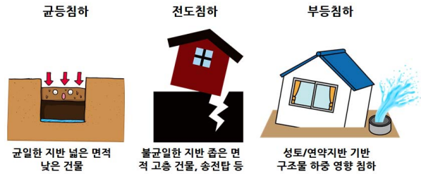
[Figure 2] Type of building settlement
