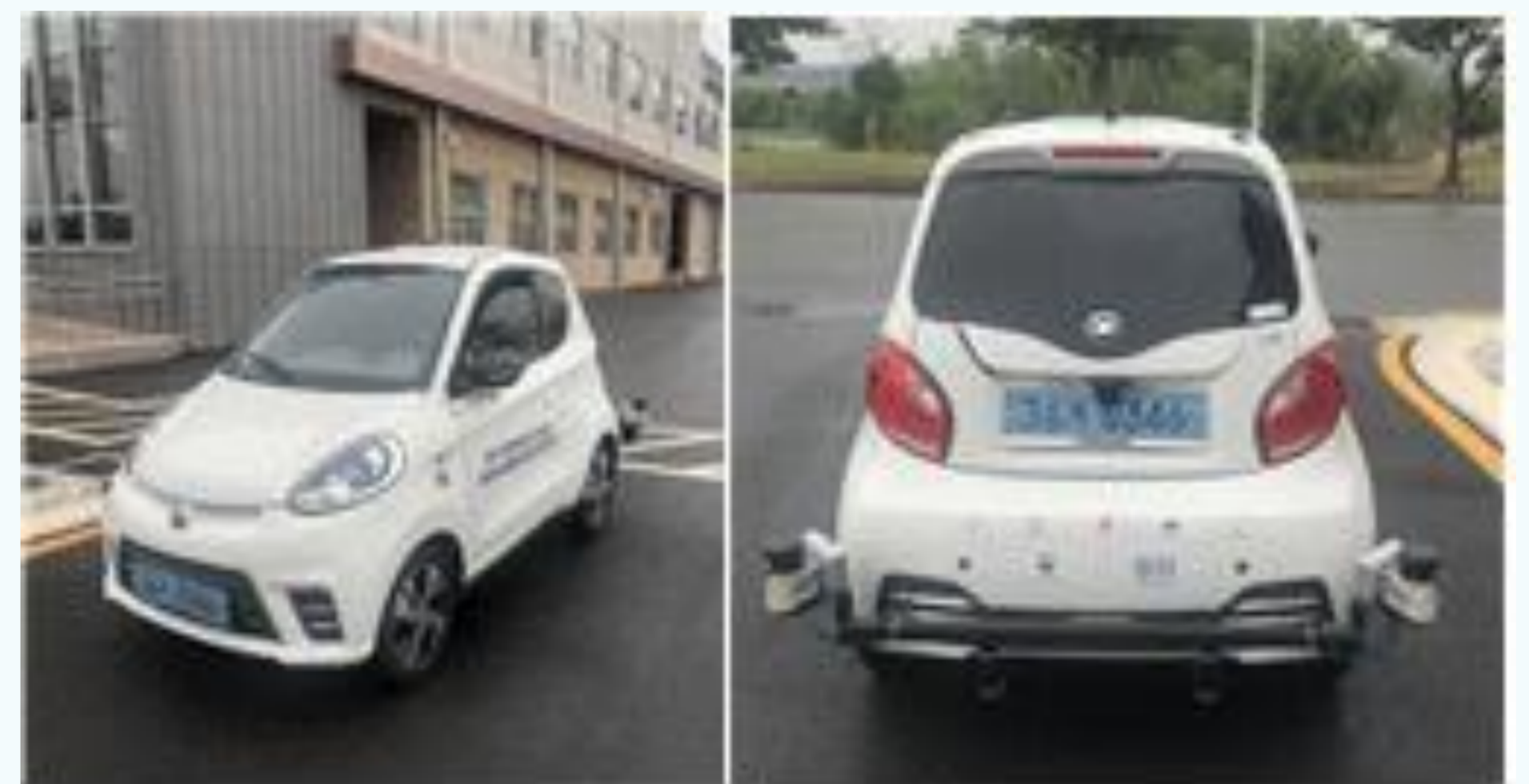
Fig. 3 SRA installed compact electric vehicle
