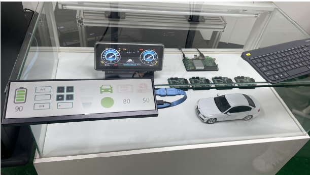
[Figure 7] OTA update scenario test prototype
